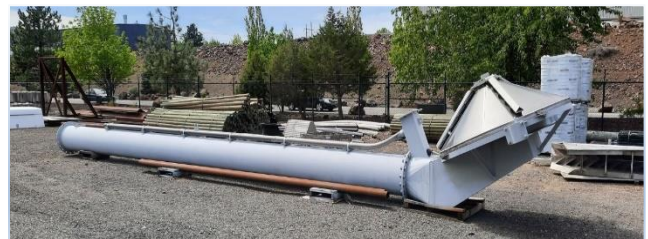
ISI C78-21 Cone Screen with 24" x 40' intake pipe
